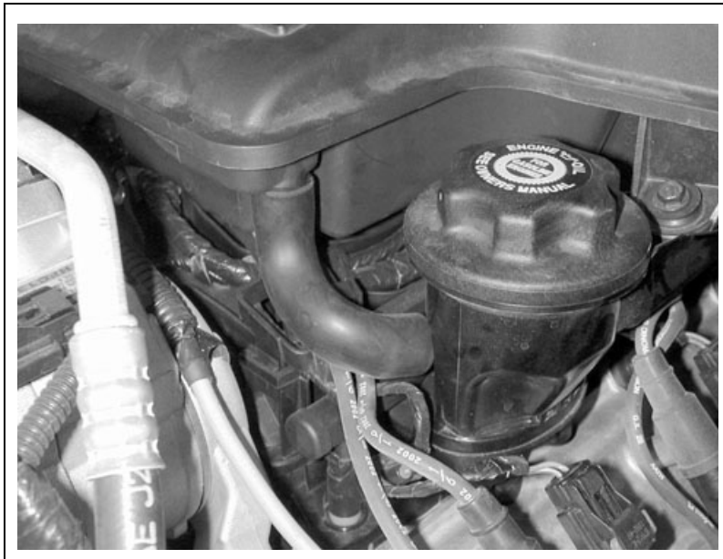
Figure 28 5.7L PCV Fresh Air Inlet Hose
