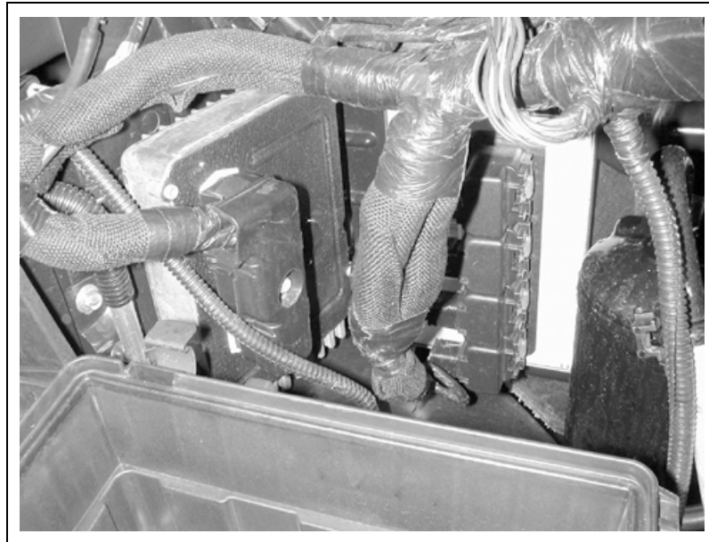
Figure 14 5.7L EATX Transmission Control Module
